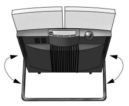
Tilt the EXPLORER<sup>™</sup> 500 slowly up or down until it points in the correct vertical direction, known as the **Elevation**. Hold the battery module and the support bracket while moving the antenna. Do not place your hands on the antenna.
