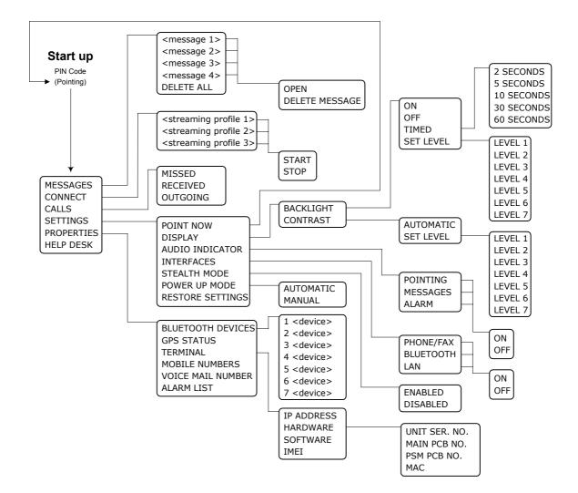
The next section shows an overview of the start-up sequence before entering the menu system. The menus are further described in the following sections of this chapter.
